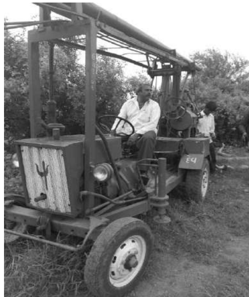
Nileshbhai Sutariya with his fully automatic double-roped pulley that can reach depths of up to 1500 feet.
