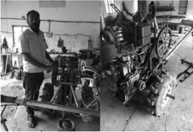
Bhaveshbhai Sutariya designed a machine with a 6.5 HP diesel engine for inter-ploughing in farms.
