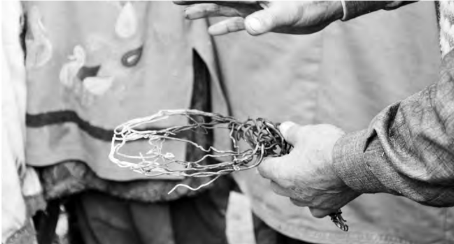
Call for redesigning: circular mesh used for cooking, often a cause for hands to burn.
