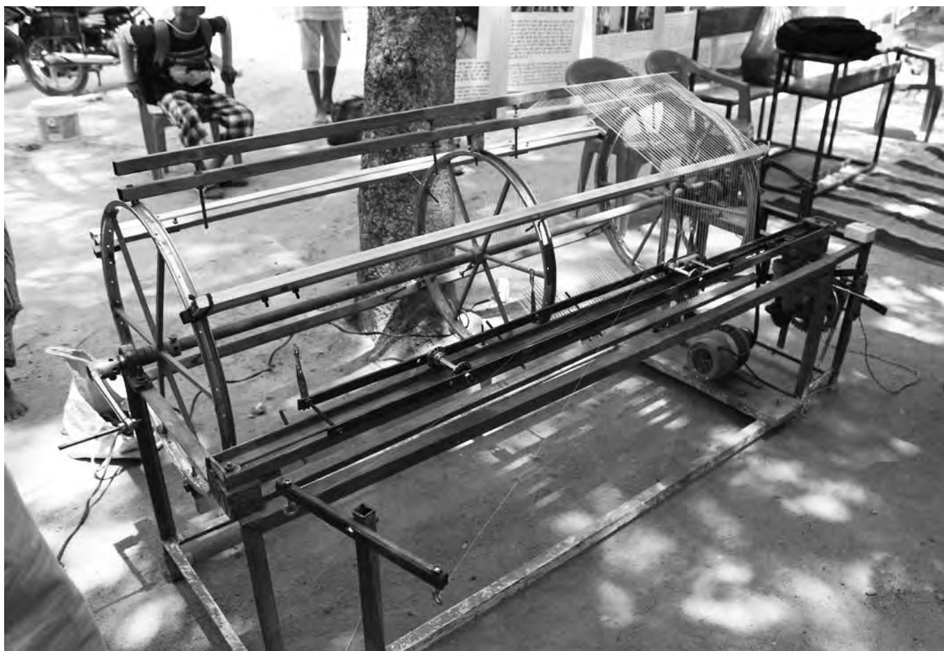
Empathy turns weaver into innovator: Multi-purpose spinning and yarn winding machine
