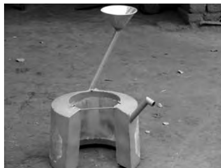
Fig 9 A double walled cooking stove
