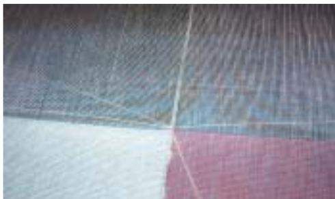
number of cones of different colours at the feeding end (selection of weft colours by dobby) a striped or checked patterns could be weaved without drop-box mechanism. For wider looms this method is very much suitable. Small sectors in the country can increase their fabric production without any additional expenses. One can weave fabrics like cotton, rayon, polyester, and silks using this method in normal plain power looms.
