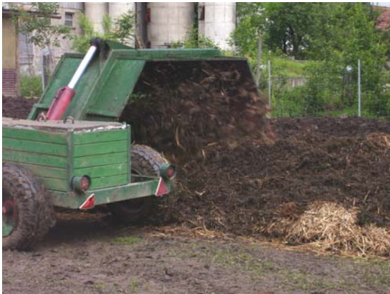
Figure 3: Compost turning machine “in action”
