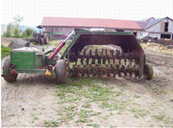
Figure 2: Self made, transportable, compost turning machine
